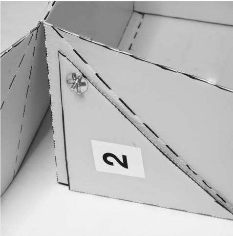
**Step 5** Now repeat steps 2, 3 and 4 on the opposite side of the cooker using panels 4 and 2. Align the holes in the panels, insert an elevator bolt from inside to outside and secure with a metal washer and wing nut, as shown in the photos above.
